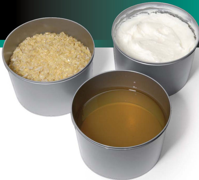
Resin, alkyd and wax compound for offset printing inks.
